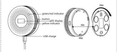
Ps1: Attach the wall plate to a groove in the back of the main engine.
